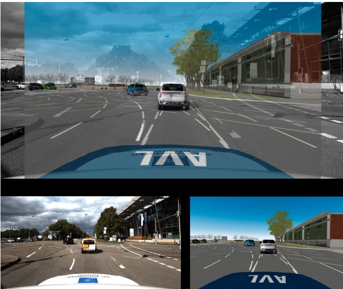
Figure 26 - Matching of digital map (static ground truth) with measured scenario (dynamic ground truth)
