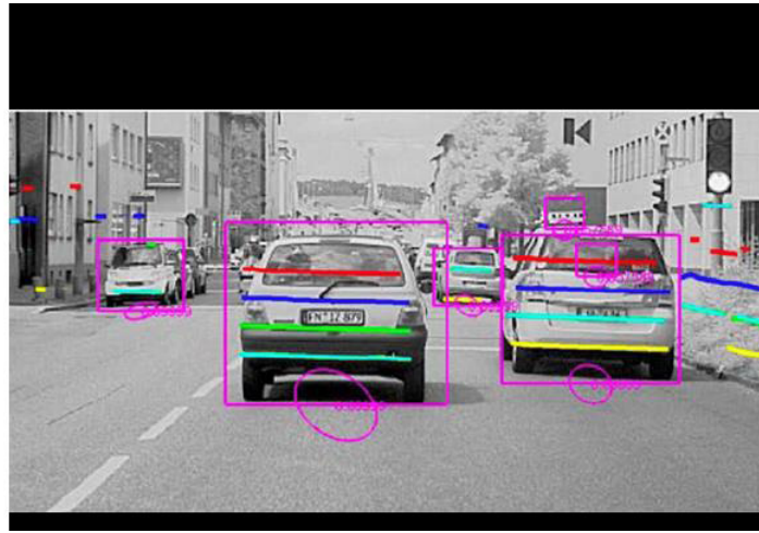
Figure33 - Detections of one and the same traffic scene as observed by Lidar and Camera
