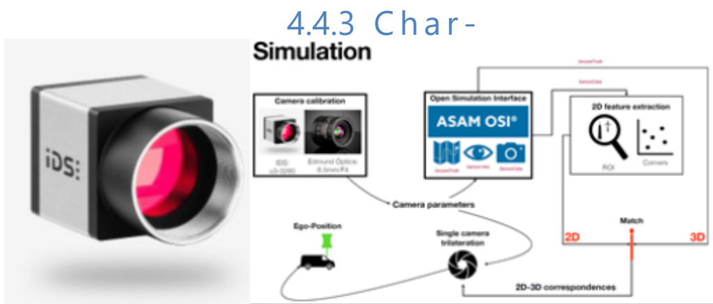
Figure 20 - The used camera IDS3280-CP (right) and an architecture of the corresponding algorithm (left)
