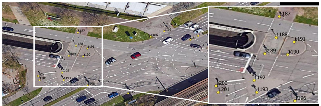
Figure 25 - Precise static measurements of landmarks as ground truth in comparison to geo referenced images (GeoTIFF)
