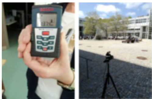
Figure 21b - Measuring the camera height (left) and taking images of the building TE in the campus courtyard (right).jpg
