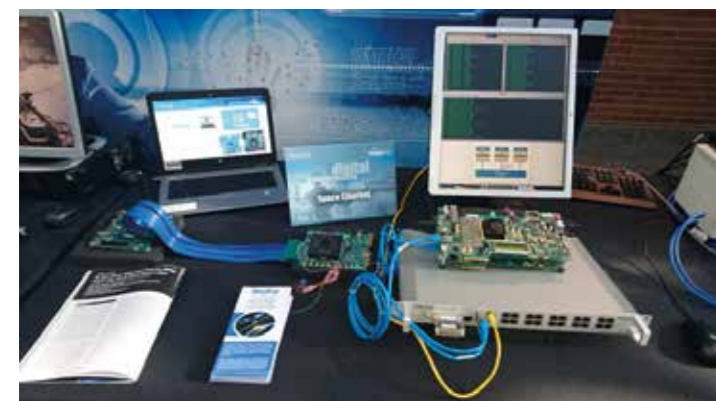
Figure 4: SEPHY Testing Setup showed at TASE Technodays in 2017, Spain. TTEthernet demonstration with three elements: FPGA with LEON 3 and TTEthernet controller, TTEthernet switch and PC with TTEthernet controller
