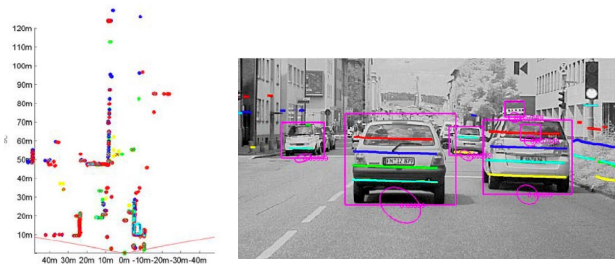
Figure 33 Detections of one and the same traffic scene as observed by Lidar and Camera
