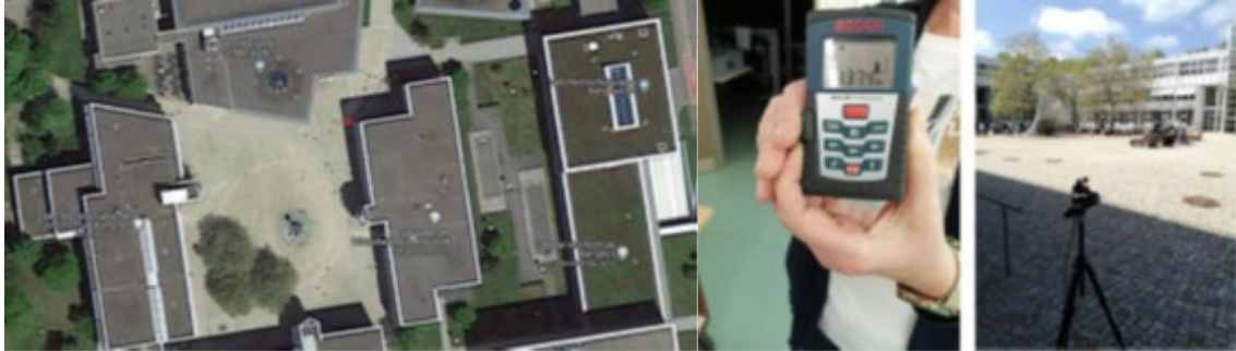
Figure 21 Position of the camera (red point) and the Campus University of Applied Sciences Kempten TE building on the left side (left figure). Measuring the camera height (middle figure) and taking images of the building TE in the campus courtyard (right figure)
