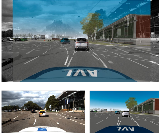
Figure 26: Matching of digital map (static ground truth) with measured scenario (dynamic ground truth)
